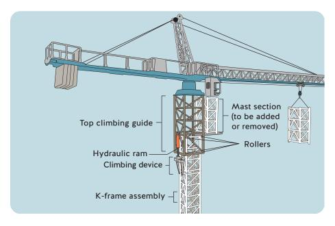
A top climbing guide is shown installed around a tower crane's mast. The guide is used to create a gap for adding or removing mast sections.
