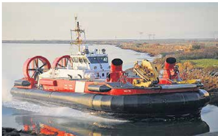
The CCGS Moytel is a British-built Griffon Hoverwork model AP1-88 Dash 400. The vessel is 26.5 metres long and powered by four Caterpillar C32 engines. Photo courtesy of griffonhoverwork.com
