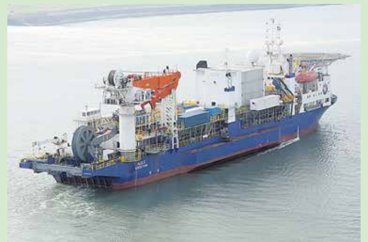
Lengkeek Vessel Engineering Inc. installed a crane on the Agile, a vessel that was converted from cable-laying to pipe-laying. Photo courtesy of Lengkeek Vessel Engineering Inc.
