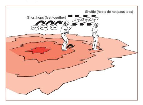
3. Continue shuffling or hopping until you are at least 10 metres (33 ft.) away. Stay further away if the voltage is over 60 kV (60,000 V) or if the ground is wet. Do not return to the crane for any reason.
