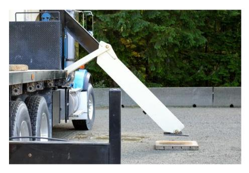
3. Extend the front outriggers onto the pads to level the crane side to side.
