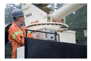
6. If the crane is equipped with a front (bumper) outrigger, extend it onto the pad. Extend the front outrigger only after the crane is levelled.
