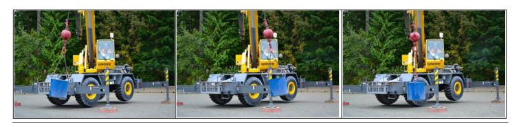
When catching a load, all crane movements during operation must be made slowly to prevent side loading of the boom.
