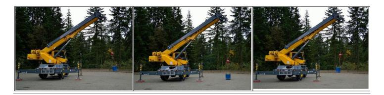
When catching a load by raising the boom, care must be taken to prevent the load from hitting the crane. You must also ensure that the swinging load is not at a radius beyond the crane's capacity.
