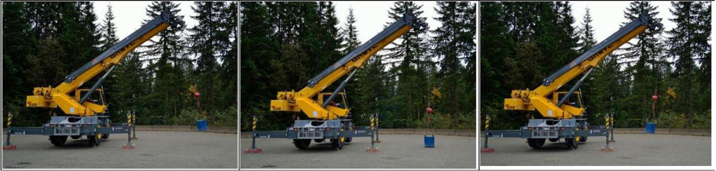
When catching a load by raising the boom, care must be taken to prevent the load from hitting the crane. You must also ensure that the swinging load is not at a radius beyond the crane's capacity.
