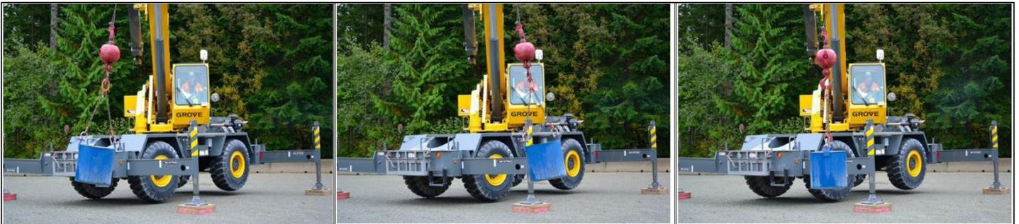
When catching a load, all crane movements during operation must be made slowly to prevent side loading of the boom.
