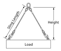
7. What is the minimum size of the two chain slings required to lift a load weighing 12,000 pounds?
